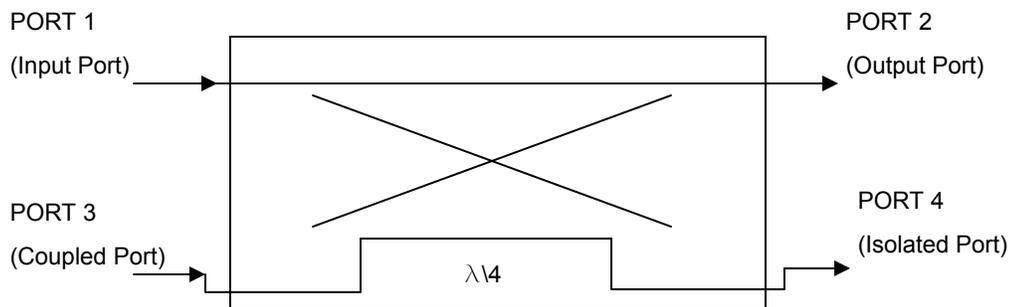
Figure 2: General layout of a coupler
