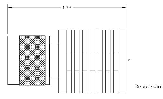
NOTE: Dimensions shown are for 5 Watt models. For 10 Watt models, body diameter increases to .99 and overall length increase \*Also available in TNC
